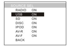
This menu can set up the above items by pressing [▲] and [▼] and ENTER. If you set one of them OFF, the function is invalid. For example, if one item set OFF pressing SOURCE button can not activate it. During playback mode, you can not set it OFF.
